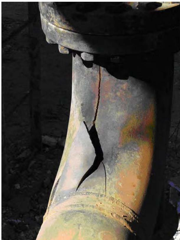
Figure 6. Crack in the 10" diameter propane mix control station inlet elbow
